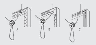
A: Fixing cords with hooks 3663 B and C: Fixing cords by using existing frame hangers Adjust and fix cord by turning the plastic screw.
